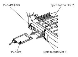
Figure 4-11 Installing and Removing a PC Card
